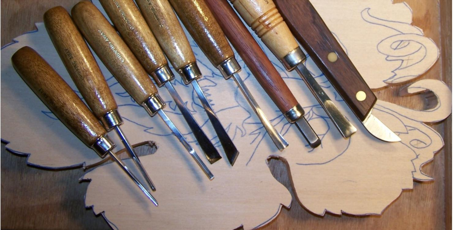
From left to right - u-gouge, micro v-gouge, v-gouge, straight chisel, skew chisel, large round gouge, bull nose chisel, wide sweep gouge, bench knife.
