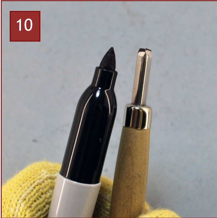
10 Remark the beveled side of the v-gouge with your marking pen.
